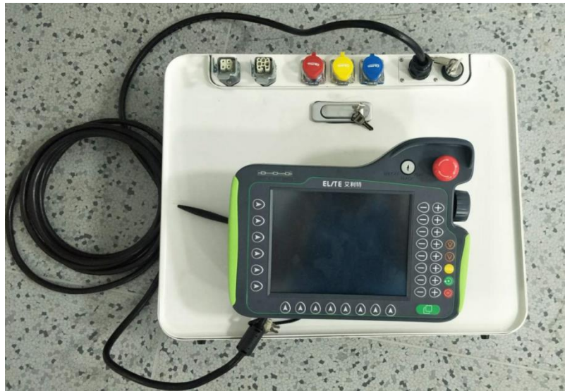
Figure 1-1 Emergency stop button
